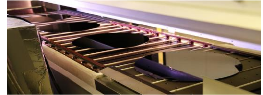
Wafer moving on ceramic rollers
