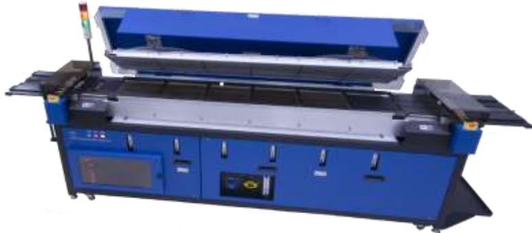
convection, the Falcon 8500 contains 1 load zone, 5 heat zones and 2 cooling zones and includes automatic load and unload buffers with appropriate sensors providing SMEMA interface connection to link into automated production lines. The system may be operated with air, nitrogen or forming gas.
