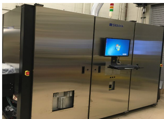
Fig. 7. EA-enabled oven for production-scale wafer bump reflow (EA UP1200 by Sikama)
