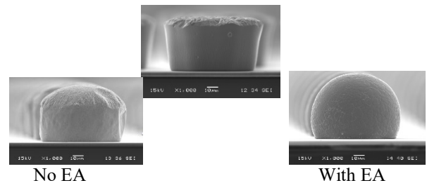
No EA With EA Fig. 6. Effect of EA on solder reflow CURRENT PROCESS STUDIES
